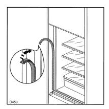
Apply covers (B) on joint cover lugs and hinge holes.
